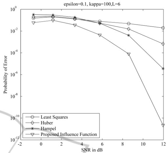
Figure 3: Probability of Error versus SNR for user 1 for linear multiuser detector, minimax detector with Huber, Hampel and proposed  $M$ -estimator in synchronous CDMA channel with impulse noise,  $N=31$ ,  $\epsilon = 0.1$ .
