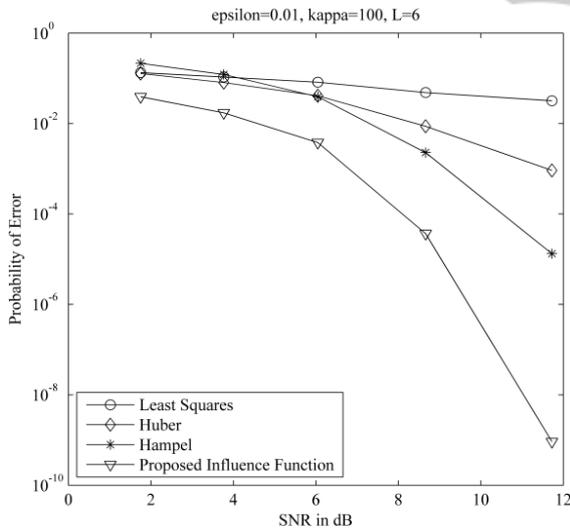
Figure 2: Probability of Error versus SNR for user 1 for linear multiuser detector, minimax detector with Huber, Hampel and proposed  $M$ -estimator in synchronous CDMA channel with impulse noise,  $N=31$ ,  $\epsilon = 0.01$ .
