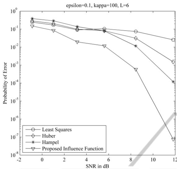
Figure 5: Probability of Error versus SNR for user 1 for linear multiuser detector, minimax detector with Huber, Hampel and proposed  $M$ -estimator in asynchronous CDMA channel with impulse noise,  $N=31$ ,  $\epsilon=0.1$ .
