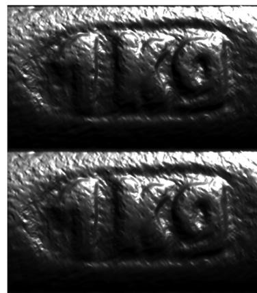
Figure 7: Full-scale synthetic image (top) and corresponding reflectance map (bottom) of the reconstructed surface. The SSIM amounts to 0.985, thus indicating a very high similarity.
