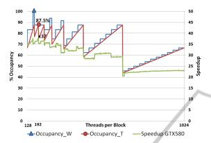
Figure 4: Analysis of GTX580 MP Occupancy and the speedup achieved with different "threads per block" values. Average values for the five test models.
