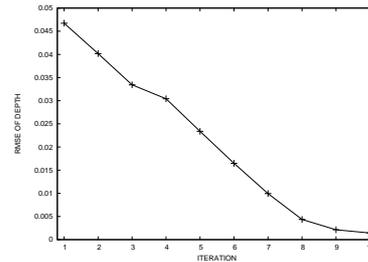
Figure 3: RMSE of recovered surface with repetition number of proposed minimization.
