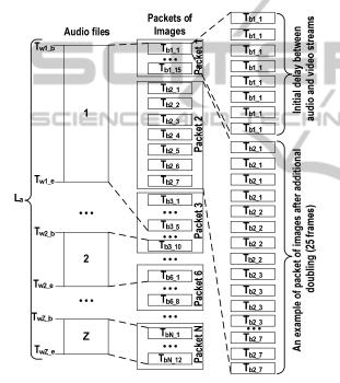
Figure 1: An example of audio and video streams synchronization for recording *avi* file.
