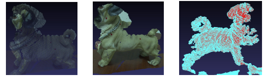
(a) Initial point cloud. (b) High resolution point cloud. (c) Two depth maps overlapped.
