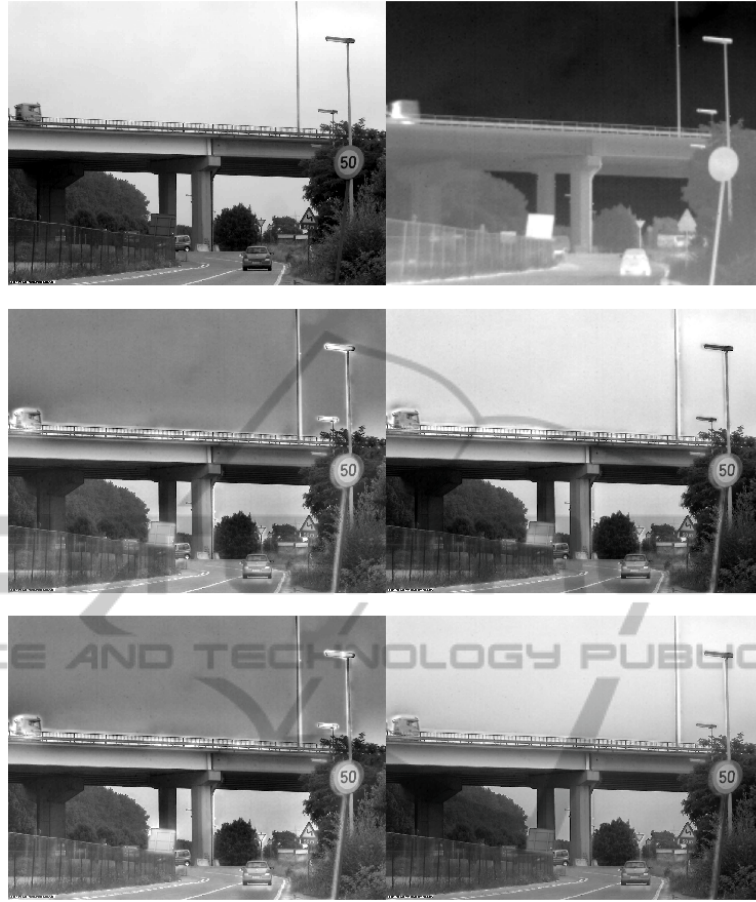
Figure 5: Top left: visual image, iconic. Top right: far infrared image. Middle left: fused image, standard fusion rule (selection). Middle right: fused image, iconic fusion rule (selection). Bottom left: Burt & Kolczynski fusion rule. Bottom right: iconic fusion rule (smooth). Top (input) images by courtesy of Xenics.
