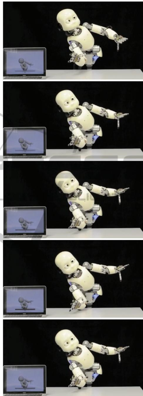
Figure 5: Time lapse images of *Virtual Skin* detecting impending collision with the table and invoking reflexive response. Collision is detected in frame 4, and response begins in frame 5.
