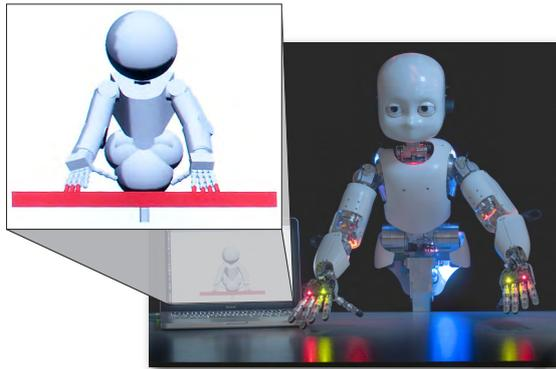
Figure 2: *Virtual Skin* detects impending collision between the iCub humanoid robot and a table. Darkened (red) geometries in the model (left) are colliding.
