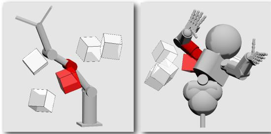
Figure 3: **Kinematic Robot Models** - The Katana arm (left) and the iCub humanoid (right) collide with random obstacles. Darkened (red) geometries are colliding.
