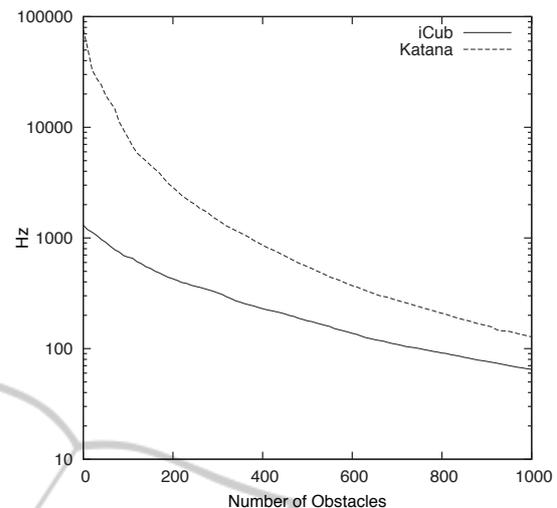
Figure 4: **Scalability of *Virtual Skin*** - A simple robot model (Katana - 9 primitives) is compared with a complex one (iCub - 129 primitives). The curves show the number of times collision detection can be computed per second (y-axis) given a particular number of obstacles modeled in the robot's environment (x-axis).
