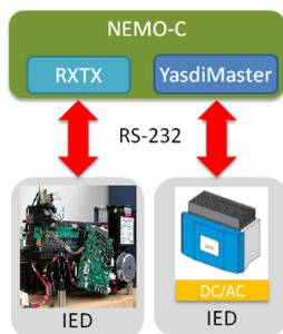
Figure 4: Fuel Cell Communication.
