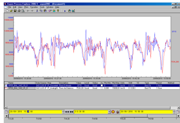
Figure 9: Comparison of actual flow and estimated flow on 09/20/2010 (Axis x = time / Axis y= flow in Ton/h).
