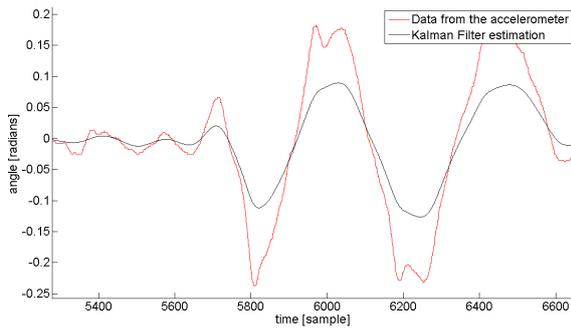
Figure 4: Measurement from accelerometer (red line) and fusion result (black line) - comparison.
