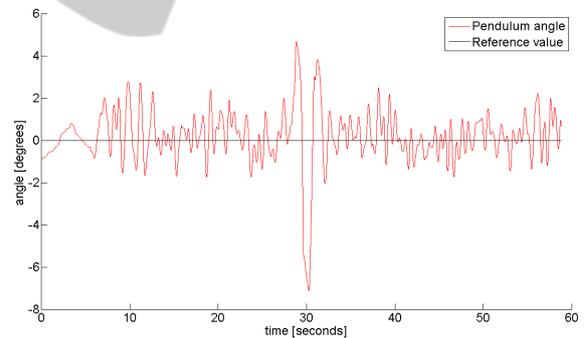
Figure 8: Experimental trajectory of the first state variable (angle from vertical position).
