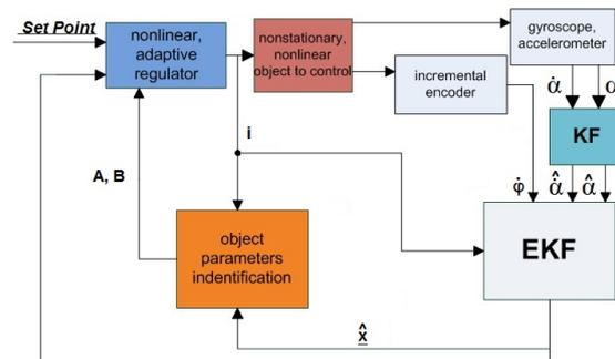
Figure 2: Overall control scheme.
