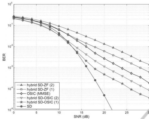
Figure 3: BER performance of hybrid SD-OSIC vs. SD, OSIC, and hybrid SD-ZF.
