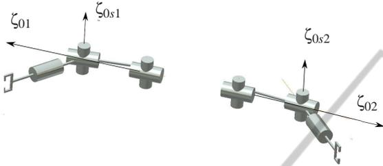
Figure 4: Constraint singularity of the dual arm system.
