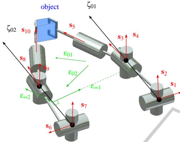
Figure 2: Reciprocal twists to parallel constraint forces (2T2R motion mode).
