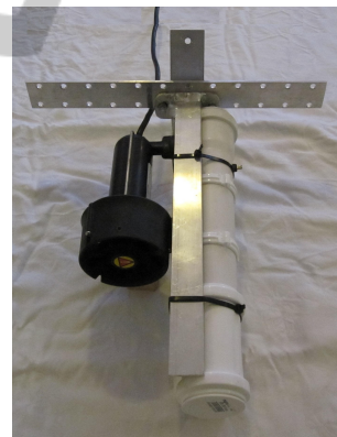
Figure 7: An assembly of the thruster, bracket and float.
