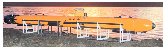
Figure 1: The Gavia AUV is commercially available and is capable of various missions, such as oceanography and pipeline inspection.
