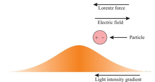
Figure 3: Schematic illustration of the transverse force in the Rayleigh regime, where dielectric particles can be treated as perfect dipoles. The Lorentz force caused by the gradient of light intensity attracts the particle towards the maximum intensity of the beam; adapted from (Schaevitz, 2006).
