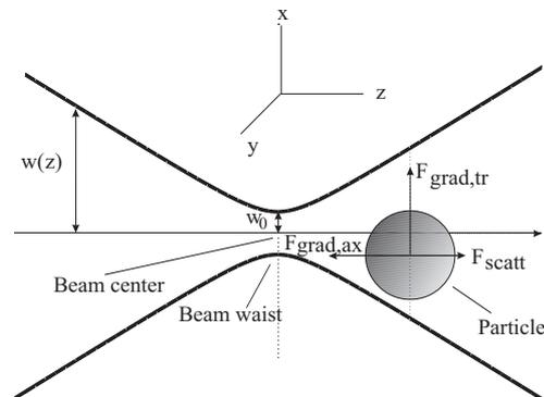
Figure 4: Modeling of trapping force exerted on particle located in a focused Gaussian beam in the Rayleigh regime.
