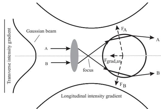
Figure 2: Schematic of a three-dimensional optical trap. The laser light is focused by a high numerical-aperture objective. The axial components of  $F_A$  and  $F_B$  add to each other and pull the sphere towards the focus forming a three-dimensional trap.
