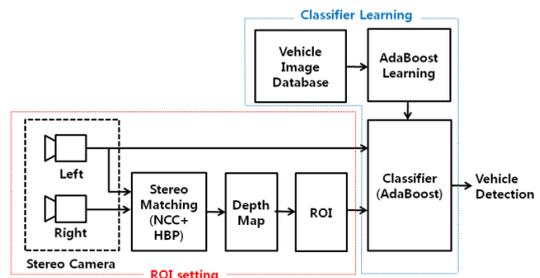
Figure 3: Stereo vision based vehicle detection.
