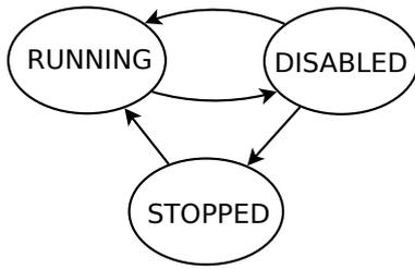
Figure 3: State diagram of a cluster computing node.
