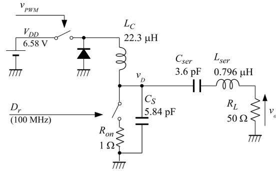
Figure 4: Simulation schematic of DC switching case. PWM pulse modulation is implemented at the drain DC bias circuits.
