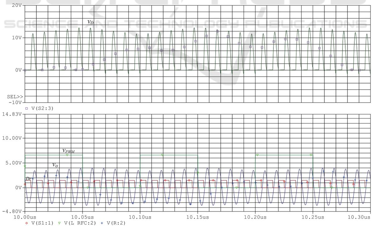
Figure 6: Simulated waveforms of DC switching case.
