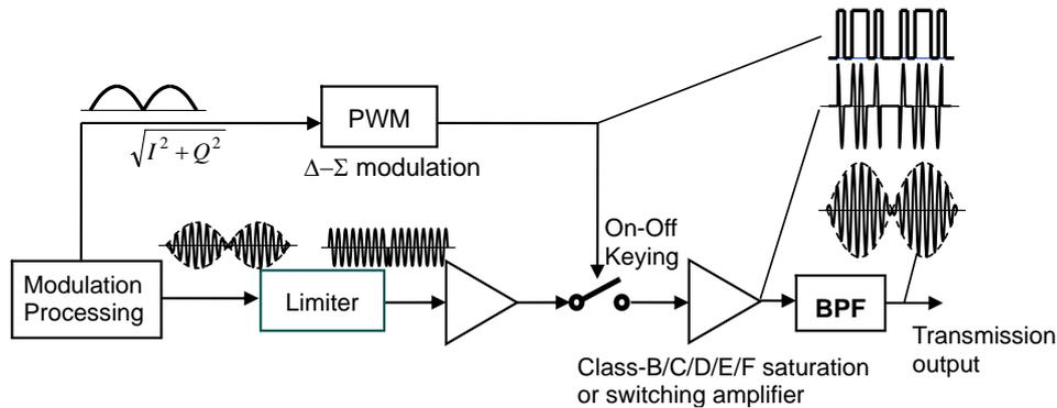
Figure 1: EDSM/EPWM transmitter
