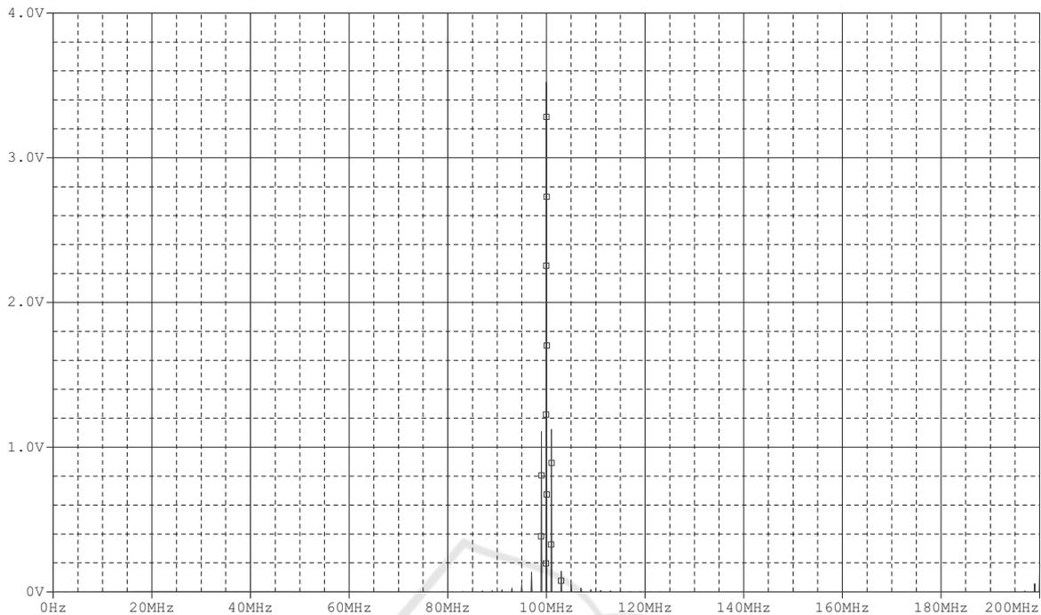
Figure 7: Output spectrum of DC switching case.
