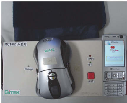
Figure 1: Three main parts of the monitor. A conventional sphygmomanometer (ABS box) with a cuff (deep blue) in the left; a mobile phone in the right; an ambulatory unit making use of a mouse crust above the ABS box.
