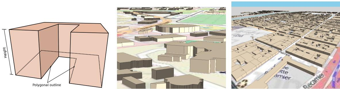
Figure 1: Figure 1(a) illustrate our building model. Figures 1(b) and 1(c) are examples of views generated by our implementation.
