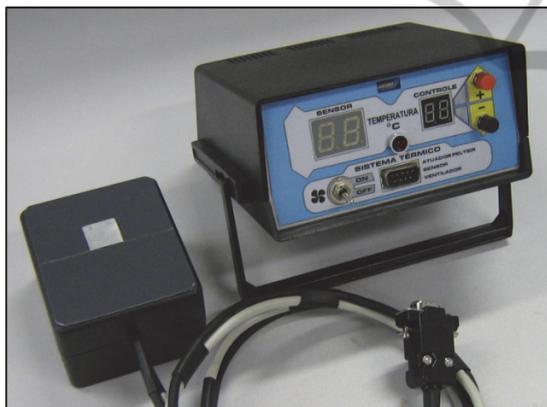
Figure 3: Portable custom built device for thermal sensitivity assessment.
