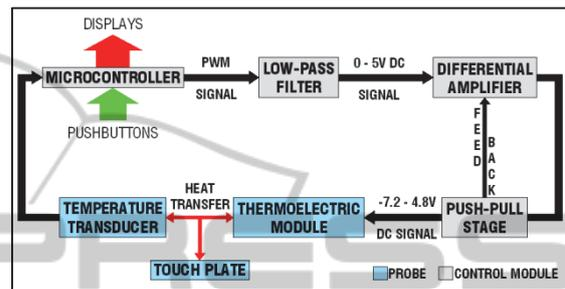
Figure 1: Block diagram of the device.
