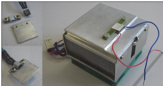
Figure 2: First stage of probe assembly.
