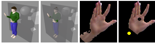
Figure 1: Hand segmentation with additional refinement. From left to right: body segmentation, original hand segmentation, hand segmentation after refinement, palm and wrist positions (black and yellow circles, respectively).
