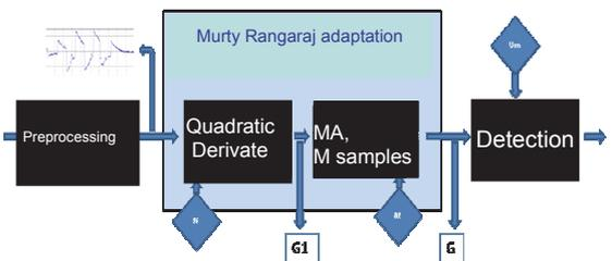
Figure 12: Block diagram of the saccade detection algorithm.
