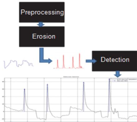
Figure 9: Block diagram of the blinking detection algorithm.
