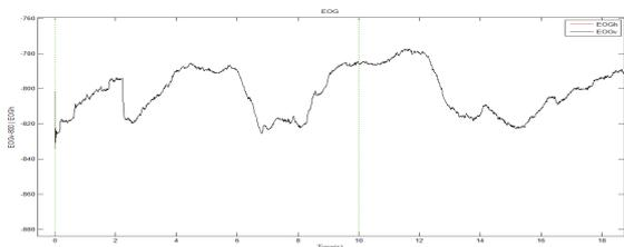
Figure 6: Seeking movement in EOGv signal. Band-pass filter 0.2-30Hz.
