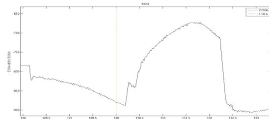
Figure 3: Compensation movement in EOGv signal. Band-pass filter 0.2-30Hz.
