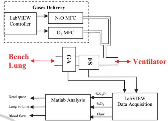
Figure 3: Layout of the Inspired Sinewave Device. The gases delivery system employs mass flow controllers (MFCs) to inject  $O_2$  and  $N_2O$  into the breathing circuit. Real-time data is read by the flow sensor (FS) and the mainstream gas analyzer (GA) and fed to LabVIEW and Matlab for estimation of dead space, lung volume and pulmonary blood flow.
