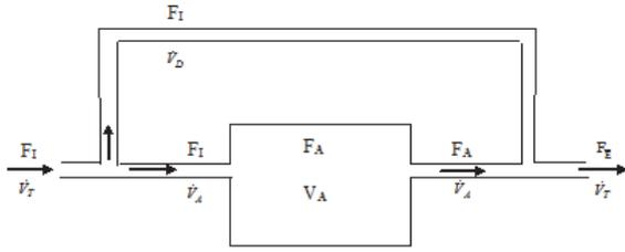
Figure 2: The continuous lung model. The inspired ventilation is branched into two parts: the alveolar ventilation  $\dot{V}_A$  which goes through an alveolar chamber, and the dead space ventilation  $\dot{V}_D$  which bypass the alveolar chamber.
