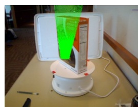
Figure 3: Planar object pose estimation using ORB.
