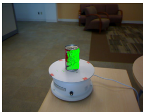
Figure 8: Non-planar object pose estimation using DARP.
