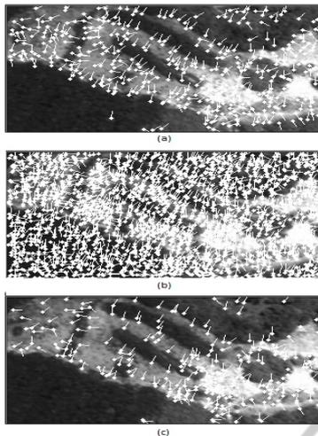
Figure 3: Keypoints detection: (a) original SIFT; (b) SIFT by DoW; (c) Our SIFT adaptation.
