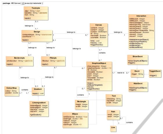
Figure 2: Class diagram of the JavaScript library that mimics the metamodel stereotypes and is used to implement the generated GUI component within a web page.
