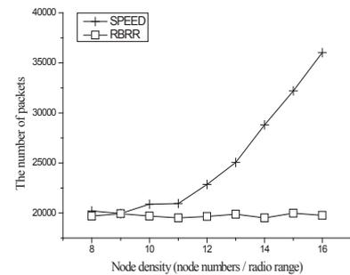
Figure 7: The number of total packets impacted by node density.
