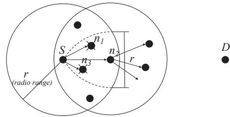
Figure 3: Basic principle of data forwarding in RBRR.
