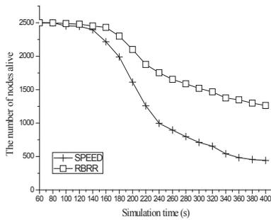
Figure 8: The number of nodes alive according to elapsed simulation time.
