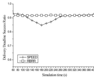
Figure 9: Delivery deadline success ratio according to elapsed simulation time.
