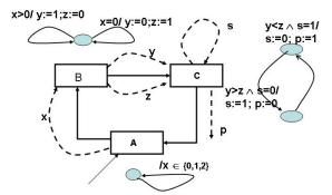
Figure 2: An RRM Diagram; C is a state holding block.
