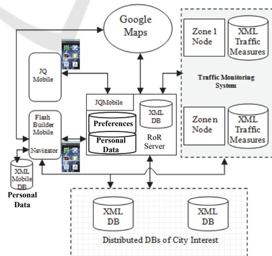
Figure 1: Wi-City functional architecture.
