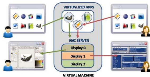
Figure 3: Application virtualization architecture.
