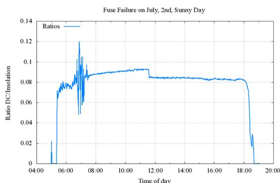
Figure 1: Plot of the DC currents curve of one inverter input, showing a failing fuse around noon on a cloud free day.
