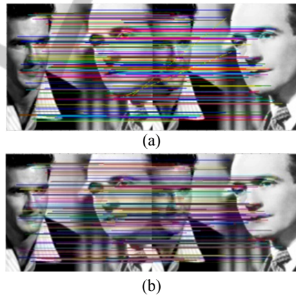
Figure 9: Example of matching between a current and desired pose. (a) Matching using RANSAC (presence of two mismatches in yellow lines). (b) Matching using PROSAC for the same camera pose.
