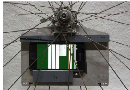
Figure 4: A Samsung Galaxy S2 as a wheel sensor at radius r_s = 9.5 cm in a bicycle wheel of radius r_w = 35 cm for data logging.
