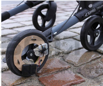
Figure 3: Prototype sensor mounted on a light-weight walker standing on cobblestone with wireless data communication.
