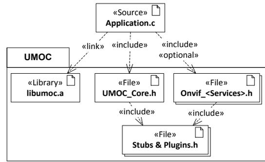
Figure 2: UMOC structure and usage.
