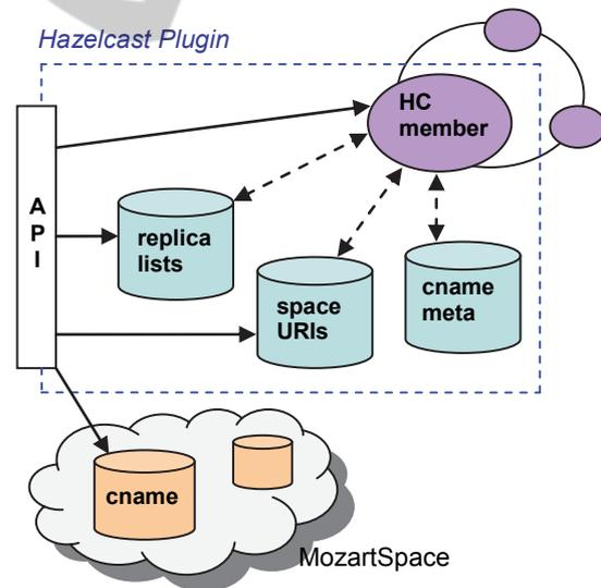
Figure 3: Hazelcast Plugin architecture (ellipses represent Hazelcast cluster members).
