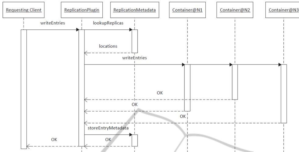
Figure 2: Sequence diagram for writing entries to a replicated container.
