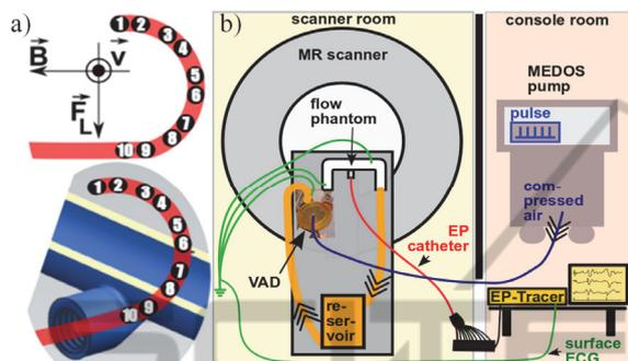
Figure 1: EP catheter positioning in the phantom and its orientation with respect to the flow velocity  $v$ , the external magnetic field  $B$ , and the Lorentz force  $F_L$  (a), and experimental setup (b).
