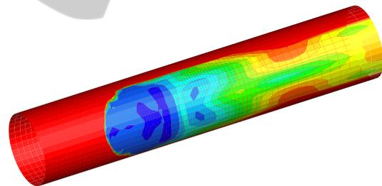
Figure 6: Axial velocity in near-wall layer.
