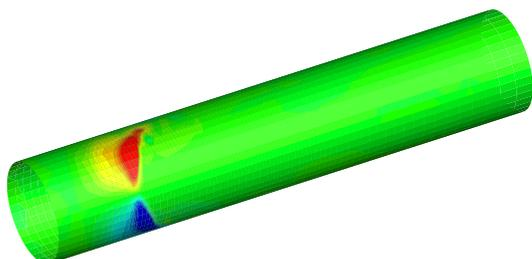
Figure 7: Tangential velocity in near-wall layer.
