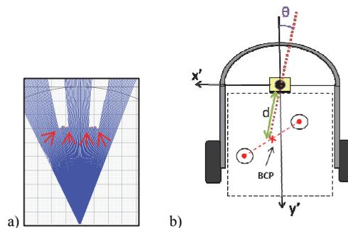
Figure 5: a) Detection of transitions: 4 transitions; b) Illustration of the CoM estimation (its location ( $x,y$ ), distance between user-walker ( $d$ ) and orientation ( $\theta$ )). the legs is calculated as the BCP position. With this information, one can know the coordinates ( $x,y$ ) of
