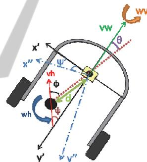
Figure 4: Scheme of the interaction parameters. Variables are defined in Table I. Black circle represents user's BCP and the yellow box represents the LRF sensor.
