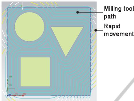
Figure 26: Generated toolpath.
