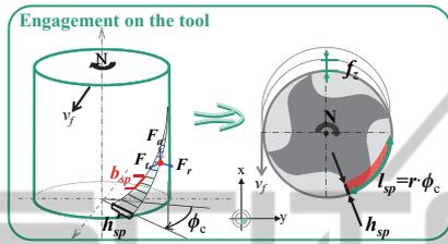
Figure 6: Engagement of cutting tool at instant  $t$ .
