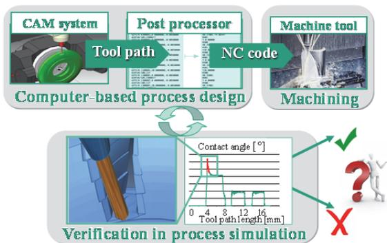
Figure 4: Evaluation of the process behaviour by the presented simulation approach.
