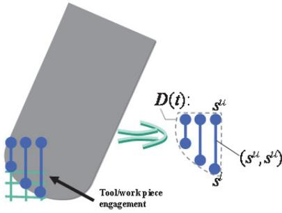
Figure 20: Set of the the intersecting dixel segments with the tool during the engagement.
