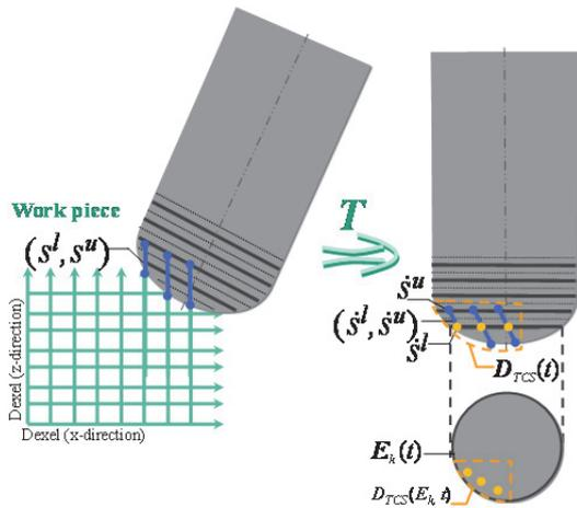
Figure 21: Material removal mapped on the discrete tool disc along the tool axis.
