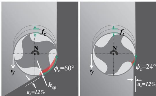
Figure 7: Straight vs. corner cuts result in different engagement despite equal cutting depth, (Diehl, 2011).
