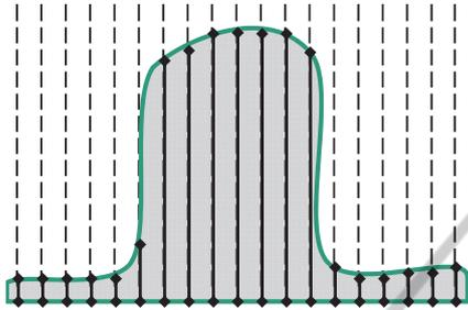
Figure 17: Dixel based representation of the workpiece.
