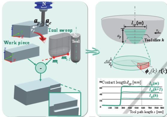
Figure 14: Geometric approach for macroscopic engagement simulation of multi-axis processes.
