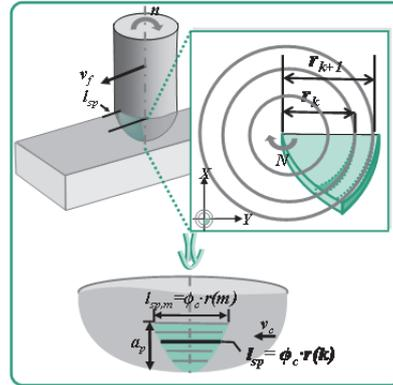
Figure 10: Influence of the tool geometry on the calculation of engagement conditions.
