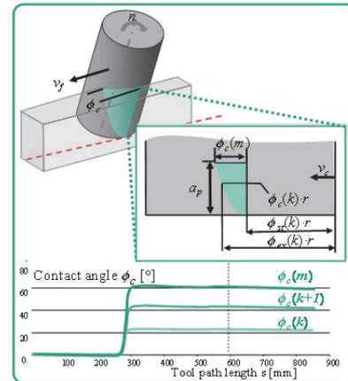
Figure 12: Influence of the tool orientation on the engagement conditions.
