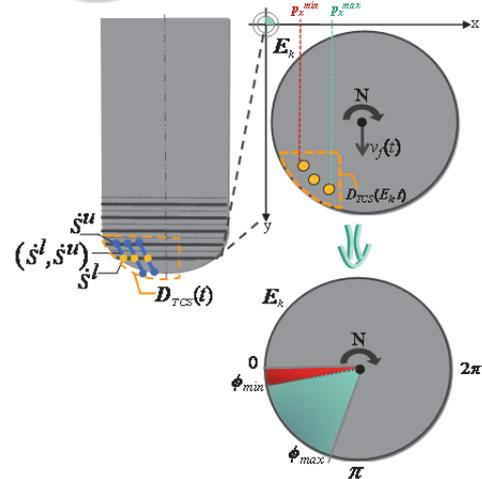
Figure 22: Estimation of the minimal and maximal angles on a tool disc  $E_k$ .
