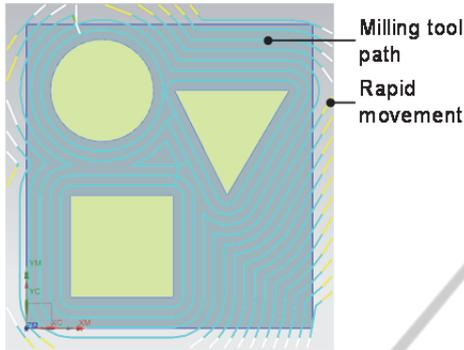
Figure 26: Generated toolpath.
