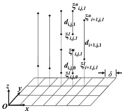
Figure 18: Logical structure of the dixel model, (Ren, 2008).
