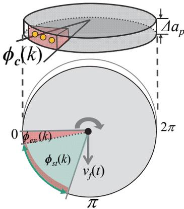
Figure 23: Calculation of contact angle on a tool disc.
