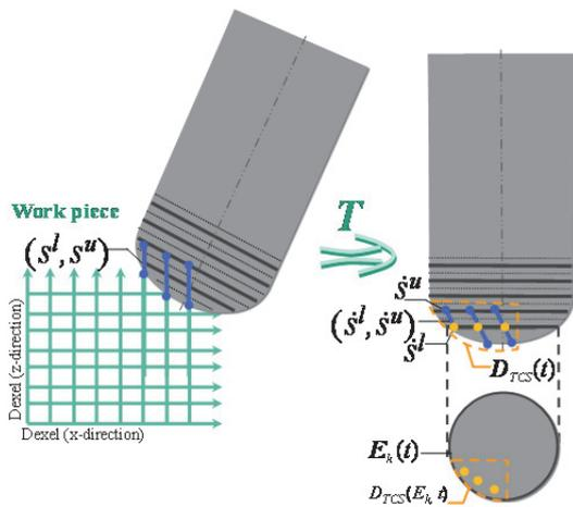
Figure 21: Material removal mapped on the discrete tool disc along the tool axis.
