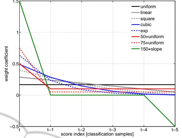
Figure 2: Comparison of the functions used for classification score postprocessing using  $k = 6$  coefficients, i.e., the current score and 5 instances back in time.
