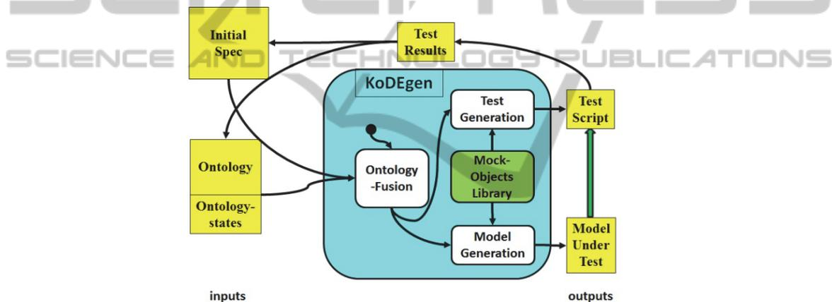
**Fig. 3.** KoDEgen Software Architecture – modules are round (white) rectangles, while inputs and outputs are regular (yellow) rectangles. Mock-Objects may complement generated code. The wide arrow upwards means that Test-Script is used to test the MUT.
