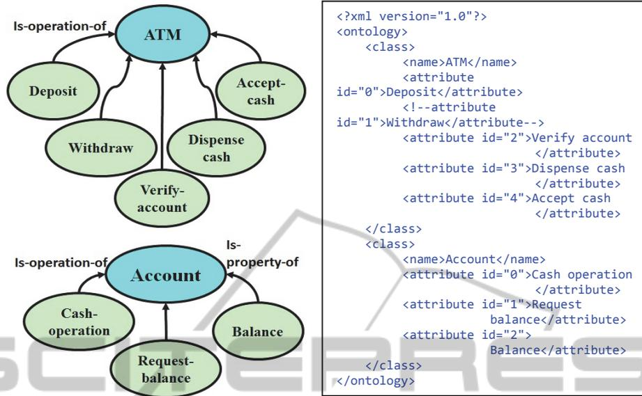
**Fig. 4.** ATM and bank Account Ontologies – A graphical representation is in the left hand side. The concepts in the ATM ontology (upper) are operations performed by the ATM. The concepts in the Account ontology (lower) are operations (Cash-operation and Request-Balance) and a property (balance) of the Account. The XML representation is in the right hand side.
