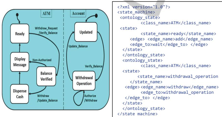
**Fig. 5.** Ontology States of the ATM and bank Account Ontology- In the left hand side the *ATM* and *account* parallel states display the states for a cash withdrawal operation. In the right hand side an XML representation for internal manipulation within KoDEgen.
