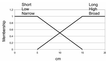
Figure 2: Fuzzy sets describing height, width and length.
