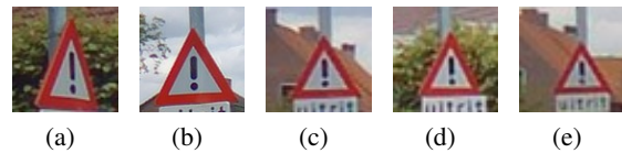
Figure 2: Example of a 3D sign, consisting of multiple detections of the same traffic sign tracked over multiple consecutive capturings.
