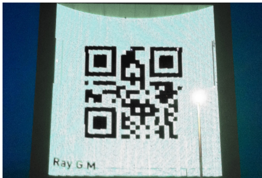
Figure 2: The curved media facade showing a QR Code that has been preprocessed using the raytracing approach.
