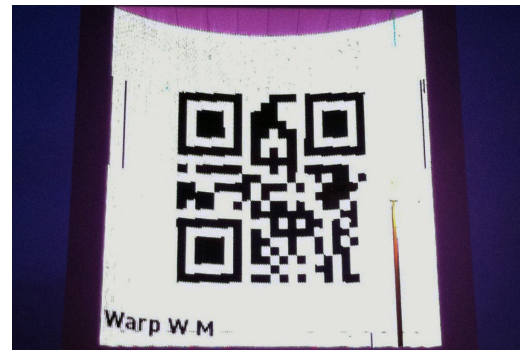
Figure 3: The curved media facade showing a QR Code that has been preprocessed using image warping.
