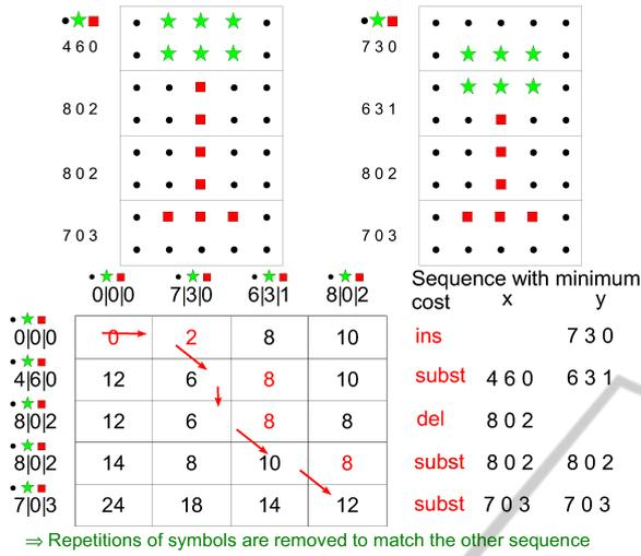
Figure 4: A toy example to illustrate the matching using SMD for the single band case.
