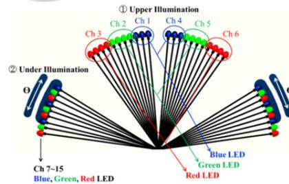
Figure 3: Structured hybrid illumination system.
