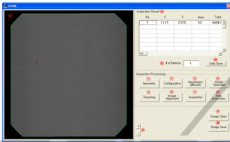
Figure 6: The inspection software.
