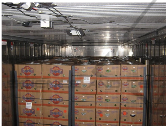
Figure 6: Pallets in test container with antennas for wireless sensors under the roof.
