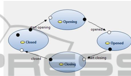
Figure 6: I/O automaton specification of a component.
