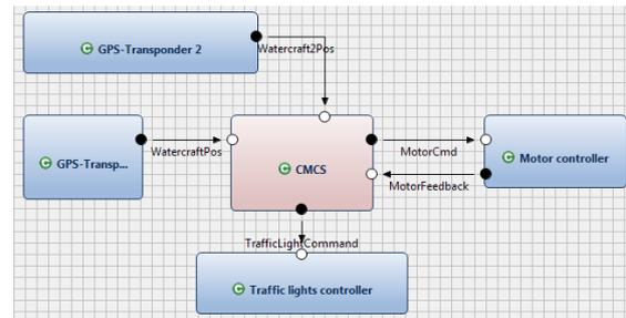
Figure 5: Example of a micro architecture specification.
