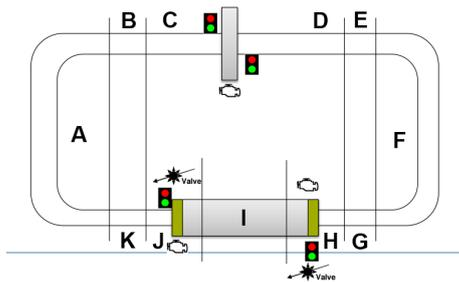
Figure 1: The topology of the canal system. There are eleven canal segments (A – K), a lock with two lock gates (bottom of the picture) and a low bridge (top of the picture). Low bridge and lock are equipped with traffic lights.
