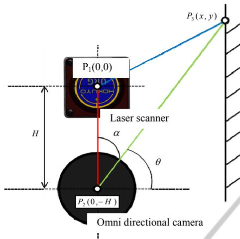
Figure 5: Relationship between omni-directional camera and laser scanner.
