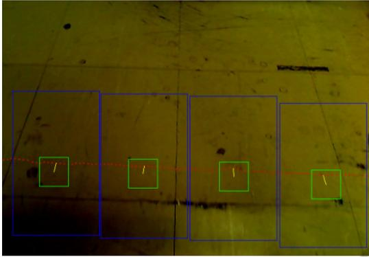
Figure 3: Detection of the movement of the cart by using optical flow.
